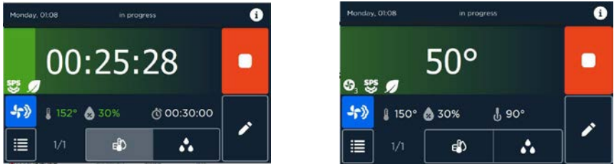
Fig. 123: Display screen Current actual values for temperature, humidity (left) and core temperature (right)
